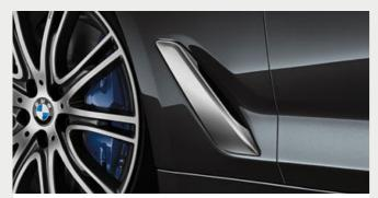
■ The Air Breathers channel air to the front wheels, reducing air resistance, fuel consumption and CO<sub>2</sub> emissions.
