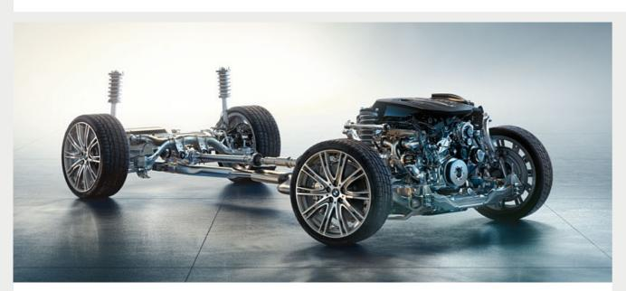
Integral Active Steering combines support that varies based on the steering angle on the front axle, and rear wheels that also contribute to steering. At lower speeds, it offers greater manoeuvrability and agility by turning the rear wheels opposite the front wheels. Beginning around 37mph, the rear wheels turn parallel to the front wheels, to increase stability and comfort.1
