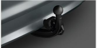
☐ The Towbar with electrically adjustable tow ball is approved for heavy loads of up to 2,000kg. In order to stabilise things, trailer stability control automatically brakes the pulling vehicle if the trailer begins to swing. The electronically adjustable tow ball is not visible when stowed under
