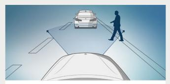
■ Person warning with city braking function actively assists the driver with the prevention of collisions involving pedestrians. It is active at speeds of up to 35mph and preconditions the brakes for increased responsiveness. In the event of an emergency, the system prevents a collision or ensures that the collision speed is considerably reduced.<sup>2, 3</sup>
