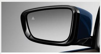
☐ If the indicator is on, the radar-based Lane Change Warning<sup>2</sup> warns the driver of approaching vehicles in the blind spot as well as vehicles in the neighbouring lane. The system functions beginning at speeds of 6mph, and in dangerous situations, it causes the steering wheel to vibrate and the triangle symbol in the exterior mirror to blink.
