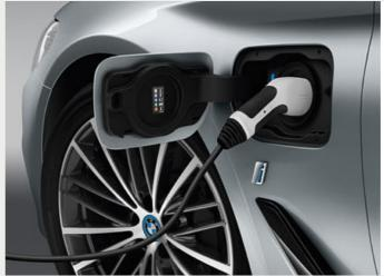
The charging port for the external charging of the high voltage battery can be found behind a flap on the vehicle's front side panel on the left. The charging port is protected from harmful environmental effects by a special gasket ring.
