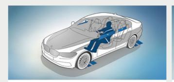
☐ **Dynamic Safety** is the BMW ConnectedDrive preventive passenger protection system. Dynamic Safety warns the driver if it detects signs of tiredness, safety belts are pre-tensioned in critical situations, electric seats are returned to upright positions and the windows and sliding roof are closed. After an accident occurs, the brakes are automatically applied until the car reaches a standstill.
