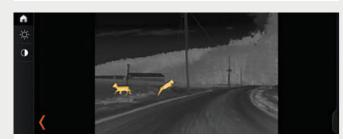
☐ BMW Night Vision with pedestrian recognition makes people and large animals visible on the Control Display from a distance using infrared imaging and illuminates them with the Dynamic Light Spot in the main headlight. An additional warning system is also automatically activated when the vehicle is started, regardless of the status of the imaging display.
