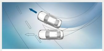
■ Dynamic Stability Control (DSC) uses sensors to constantly assess the vehicle's movements, optimising directional stability and traction by intervening in engine and brake management. This increases driving safety.
