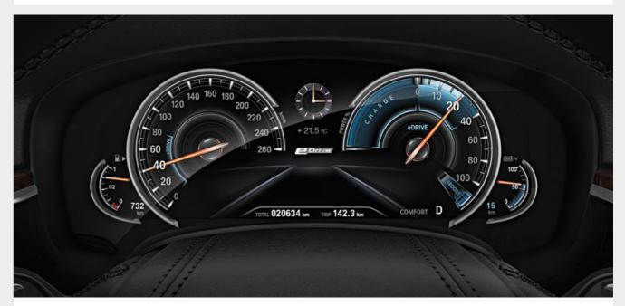
The instrument cluster includes dials that help the driver to make particularly efficient use of the electric drive with information such as battery charge level and drive status.
