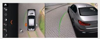
☐ Parking Assistant Plus makes parking and manoeuvring the vehicle easier. It features Surround-view including Top-view, Remote 3D view, Panorama view, PDC and Park Assist with linear guidance, which parks the vehicle parallel or perpendicular to the lane completely automatically. The system works by measuring potential spaces while driving past at a low speed.
